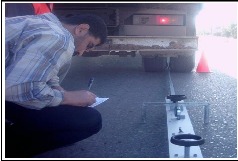
Figure (2.5): Use Benkelman device [16]
