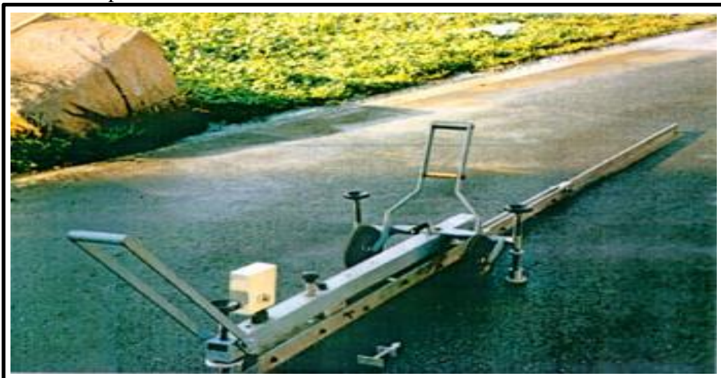
Figure (2.4): Benkelman device [16]
